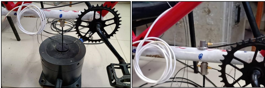
Figure 6. Shaker (left) and details of force and vibration transducers (right).
