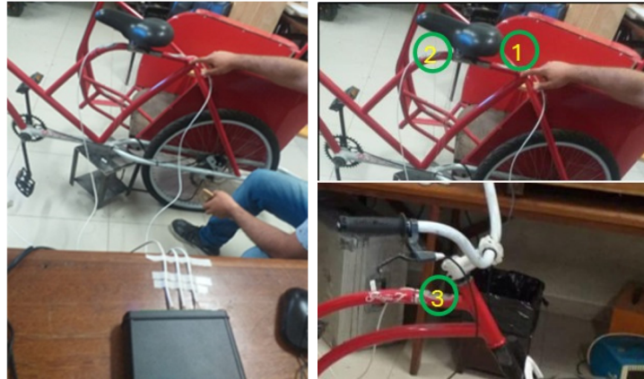
Figure 17. Use of strain gauges for numerical model validation (left) and their positions on bicycle (right).
