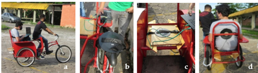
Figure 10. Measurements of whole-body vibrations: (a) measurement during bike rides; (b) sensor placed on saddle; (c) sensor placed on passenger seat; (d) sensor placed on sidecar backrest.
