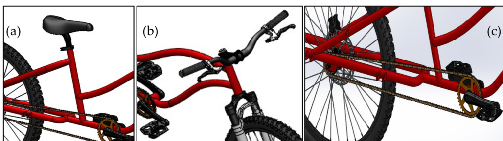
Figure 27. Bicycle details: (a) adjustable seat; (b) standardized handlebars; (c) new mechanical transmission.
