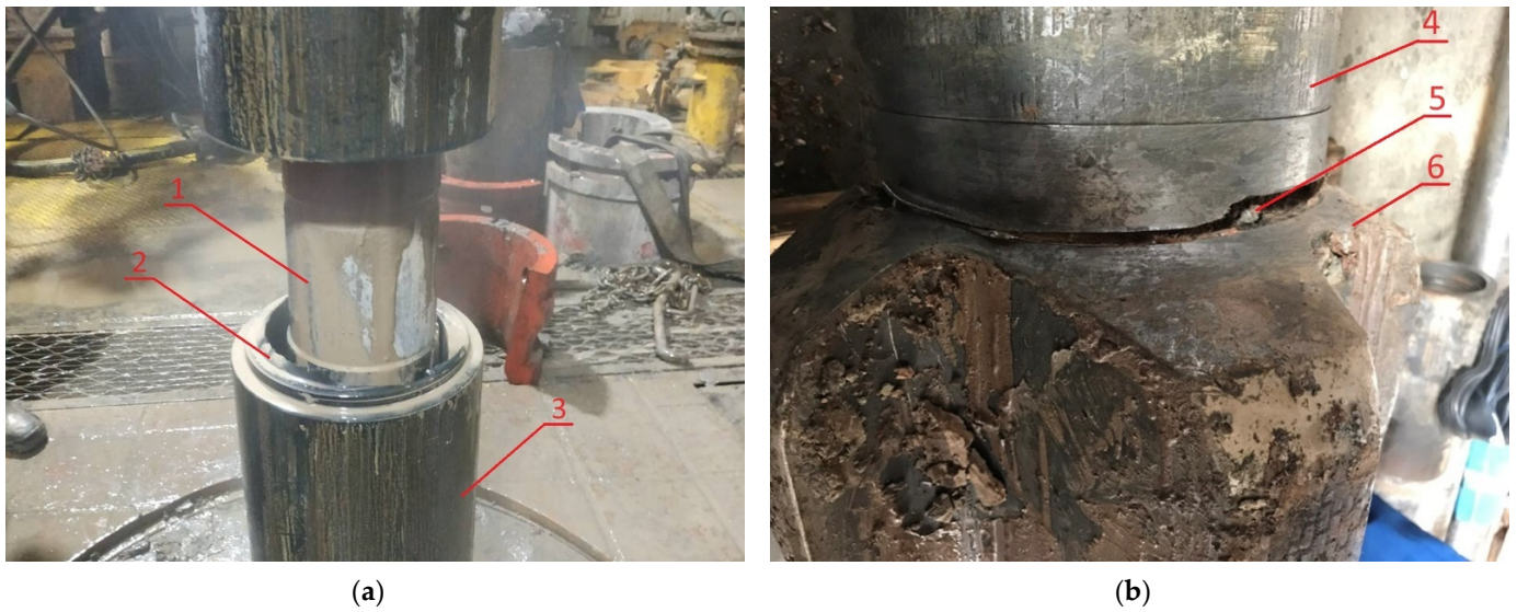
Figure 7. A visual inspection of the damage to the PDM caused by the influence of torsional vibrations: (a) Lifting a damaged downhole screw motor; (b) Destroyed stabilizer housing; 1—the rotor of the power pair; 2—the place of the fracture of the threaded nipple of the angle regulator adapter; 3, 4—PDM housing; 5—the location of the housing stabilizer fracture; 6—stabilizer blades.
