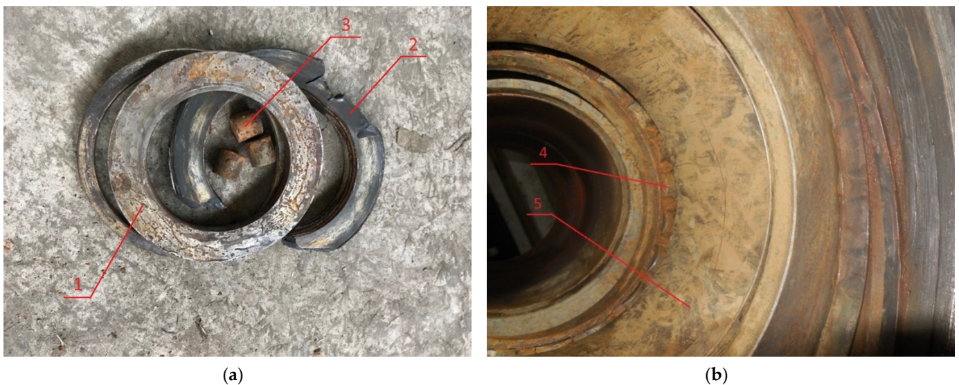
Figure 3. Damage to thrust-bearing separators and internal elements of the spindle section of the screw engine: (a) Damaged elements of the downhole motor; (b) Inspection of the spindle part of the downhole motor; 1 and 2—upper and lower bearing brackets; 3 and 4—bearing rollers, 5—PDM bearing housing.
