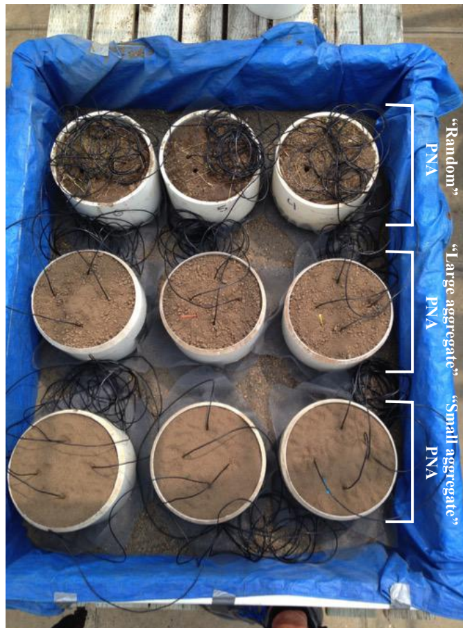
Figure S1. Experimental set up, consisting of 9 PVC rings filled with soil and instrumented with Pt-electrodes in a fiberglass tub. Treatments are Random (top row, n=3), Large Aggregate (center row, n=3) and Small Aggregate (bottom row, n=3). Blue tarp liner for easy removal of autoclaved sand.
