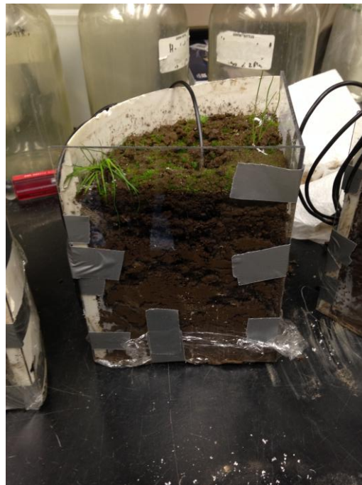
Figure S3. Sub sampling process. Panel a shows the PVC ring itself being cut. Panel b shows one of the sub samples ( n = 27 ) created from the larger PVC rings ( N = 9 ) using acrylic glass panels to create isometric subsections for subsequent XCT analysis. The Pt-electrode was kept at the center of each sub sample to maintain sample integrity.
