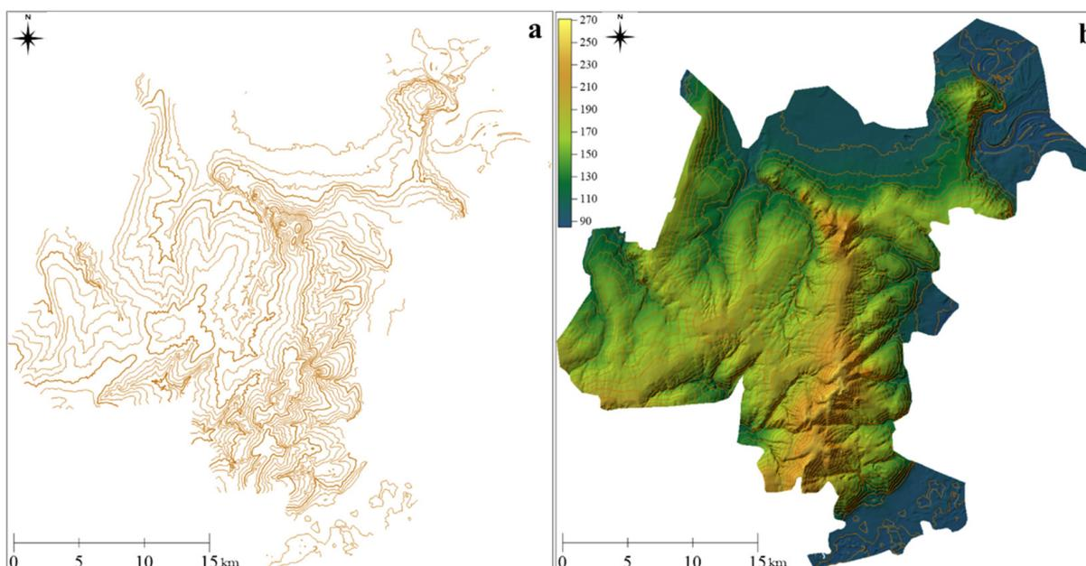
**Figure 3.** Digitized contours (a) and DEM, m (b) of the study area.
