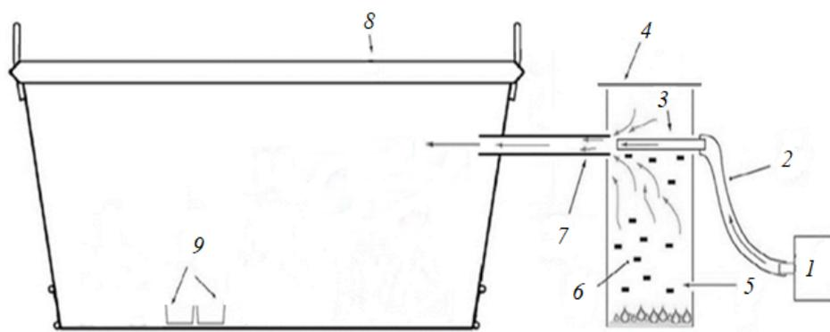
**Figure 2.** Scheme of the installation for soil fumigation: 1—Hailea ACO 208 air compressor; 2—hose from the air compressor for air supply to the smoke generator; 3—tube for air supply to the chimney; 4—Merkel Standart smoke generator; 5—holes for ignition of combustion materials; 6—smoke from thermal destruction of combustion materials; 7—chimney for smoke supply to the gas chamber; 8—gas chamber; 9—soil samples.
