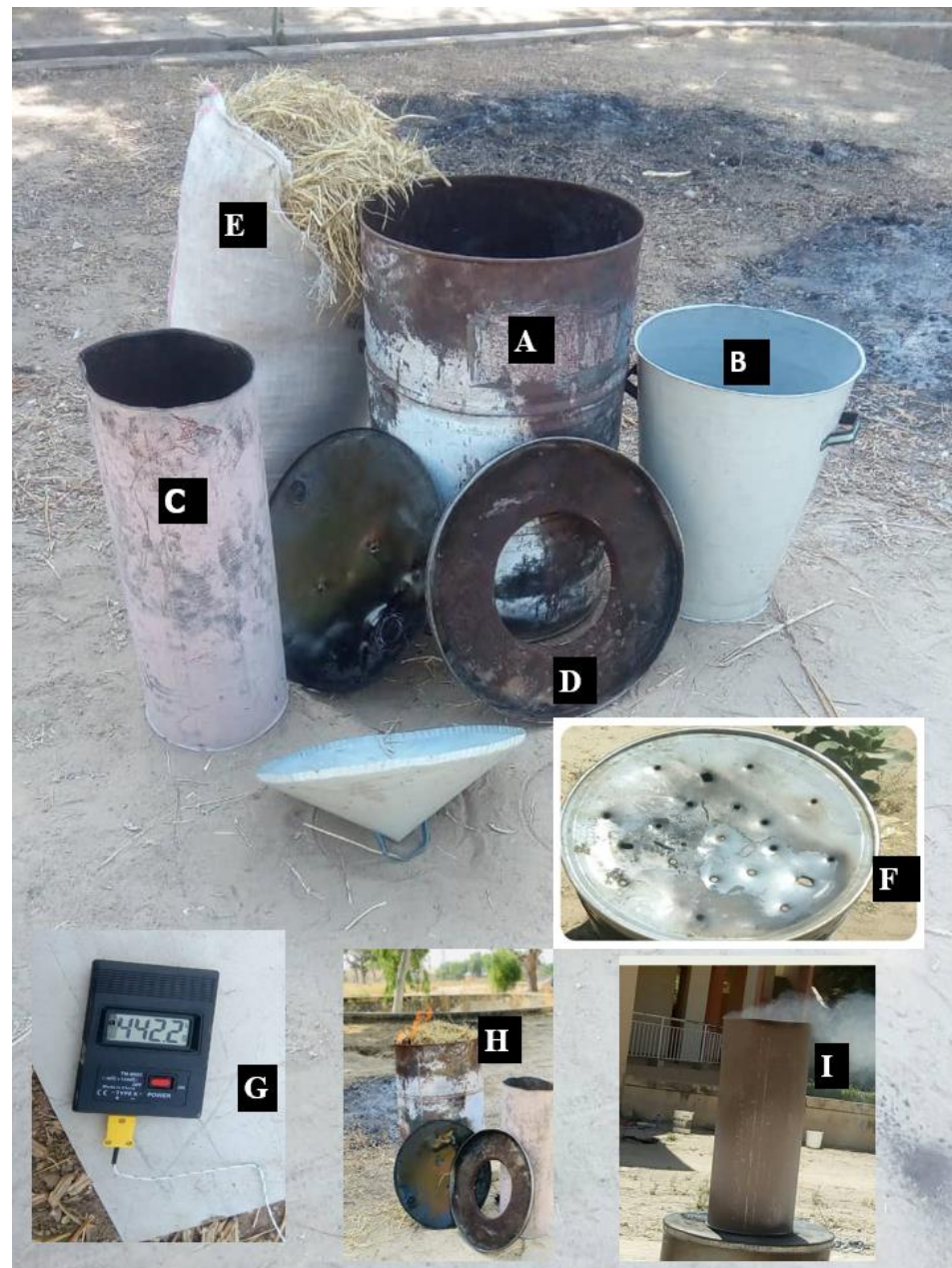
Figure 2. Local BC kiln designed by Bababe et al. [72] (unpublished): (A) drum kiln, (B) inner kiln, (C) chimney column, (D) drum kiln lid, (E) feedstock, (F) drilled holes, (G) digital electronic-probe thermometer, (H) ignited feedstock loaded in the drum kiln, (I) fixed chimney.
