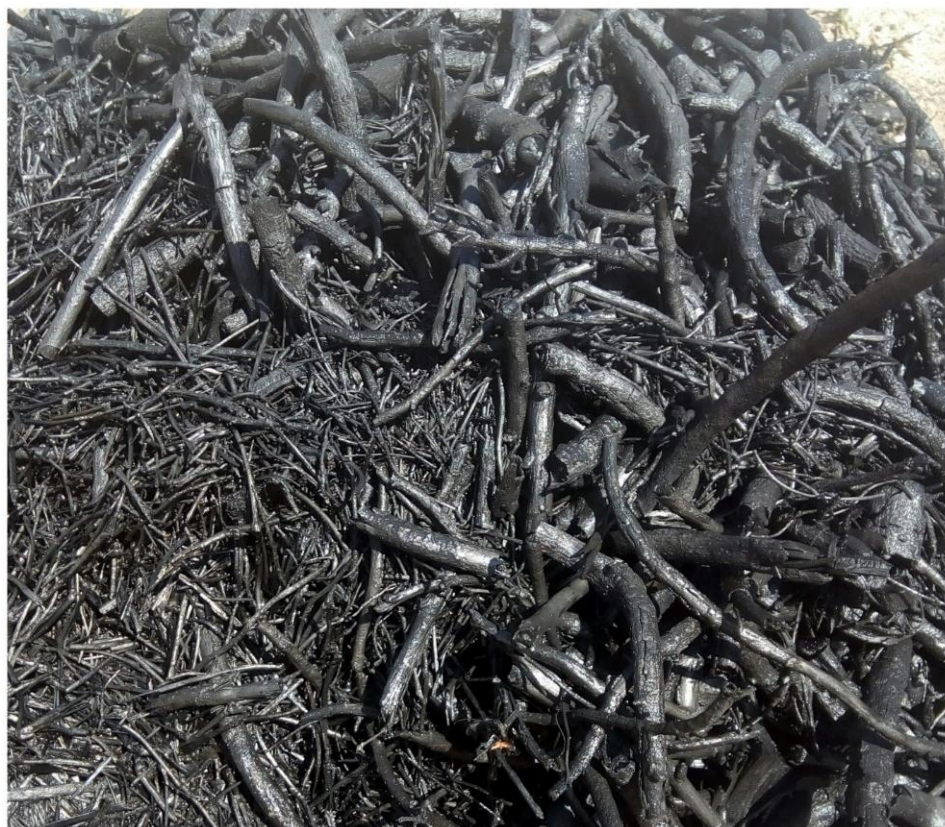
Figure 3. BC obtained from the kiln developed by Bababe et al. [72] (unpublished).
