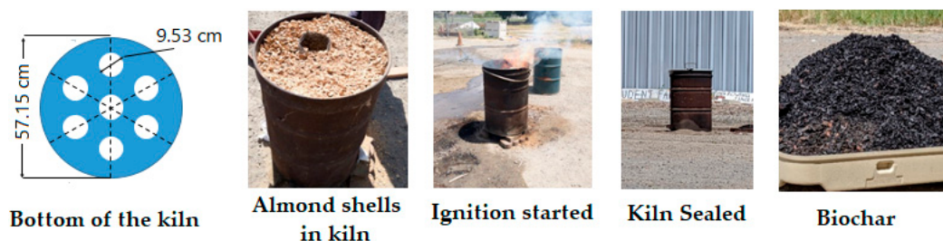
Figure 2. Production of biochar in fixed-bed pilot-scale kiln.
