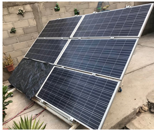
Figure 7. Partial shading artificially created with canvas.
