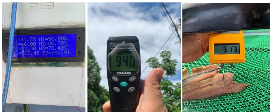
Figure 2. Data recorded using the sensor (left), solar radiation measured using a hand-held solar meter (middle), and fish moisture measured using a portable meat moisture meter (right).
