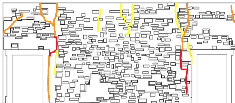
Figure 5. Map of existing cracks on the foundation wall. Red indicates cracking over 1 cm; yellow indicates cracking on the order of 1 mm; orange indicates cracking in between these two limits.
