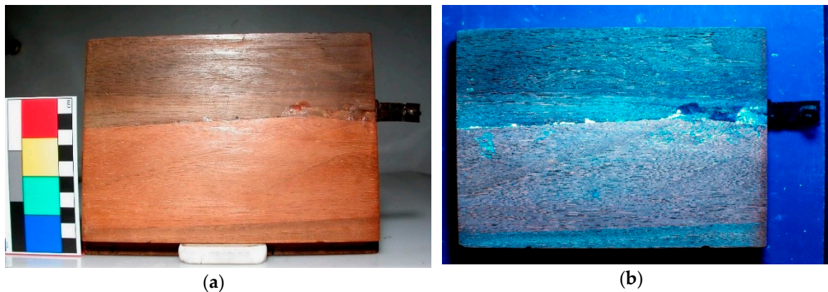
Figure 7. (a) The lid's inner side under visible light; (b) under Wood's light.
