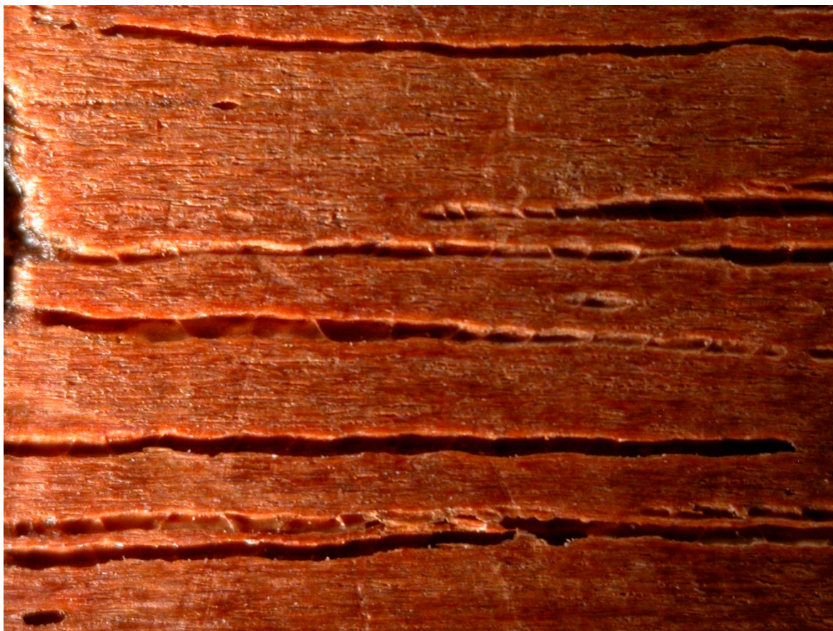
Figure 14. Enlarged detail (30×) of the longitudinal surface. Simple perforations of the transverse walls of the conductive tissues are clearly visible.
