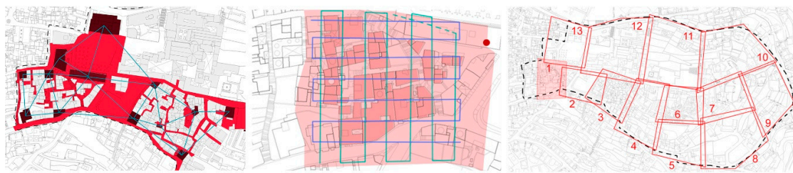
Figure 12. Project approaches for spatial control in survey campaigns, tested on the Al-Anatreh district, with a Terrestrial Laser Scanner (data acquired from streets, stairways, and keypoints of coverage level), aerial photogrammetry by drone (with grid plans of acquisition trajectory for the drone flight), and close-range photogrammetry (acquired from the ground level while considering the surface organization of aggregate and building units).
