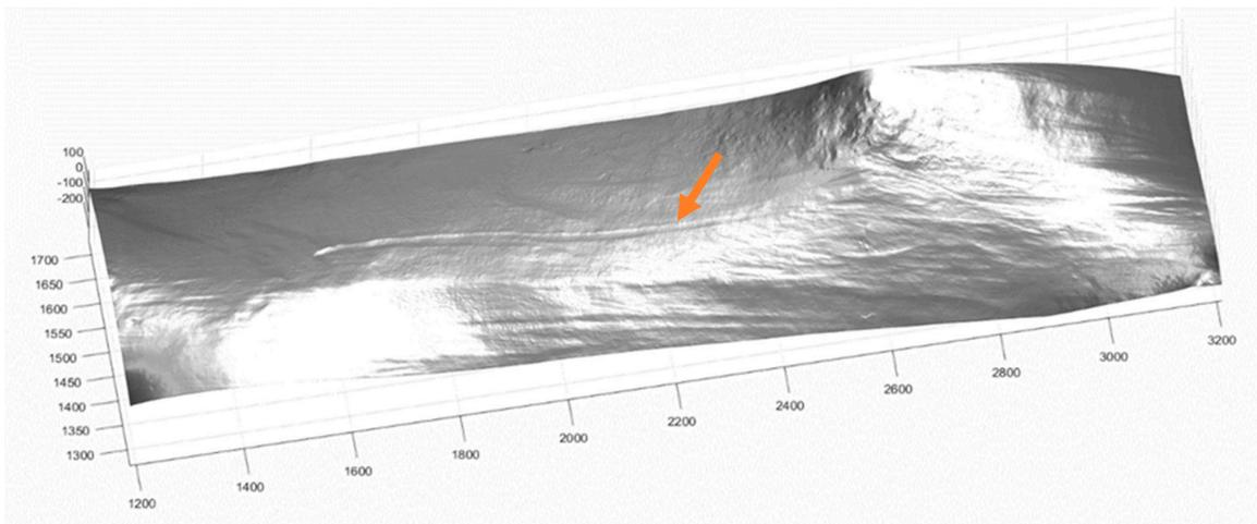
**Figure 8.** 3D reconstruction of the wood surface. The red arrow identifies the point where the surface scratch depth profile was reconstructed.
