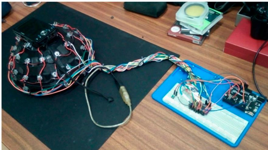
**Figure 4.** The Reflectance Transformation Imaging (RTI) instrument used in this work.
