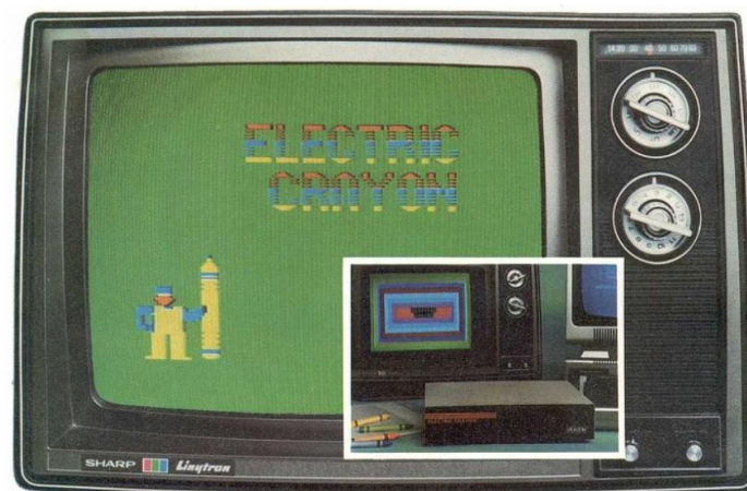
Figure 7. The Electric Crayon was $249.95 (April 1980). It was delivered complete with the EGOS system, 1 KB of video memory, and a thick user manual. Source: Internet Archive (1980) [34].
