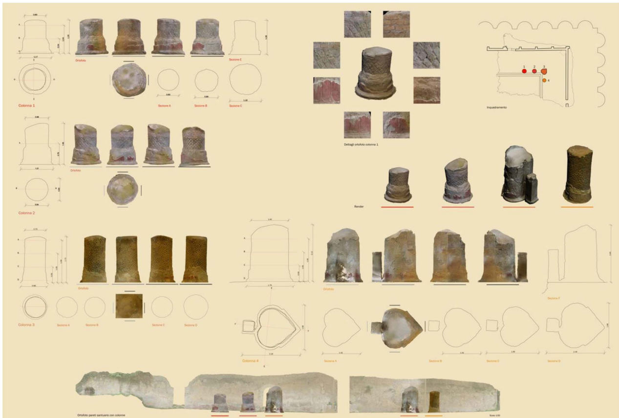
Figure 4. Final technical drawings (plans, sections and elevations) at the appropriate scales for the conservation project.
