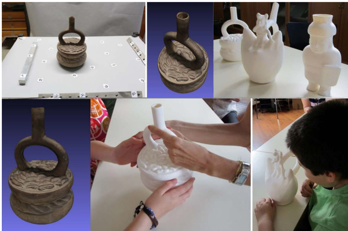
Figure 10. Activities carried out during a student stage: artefacts surveying and 3D printing to design a tactile museum route for visually impaired or blind people.
