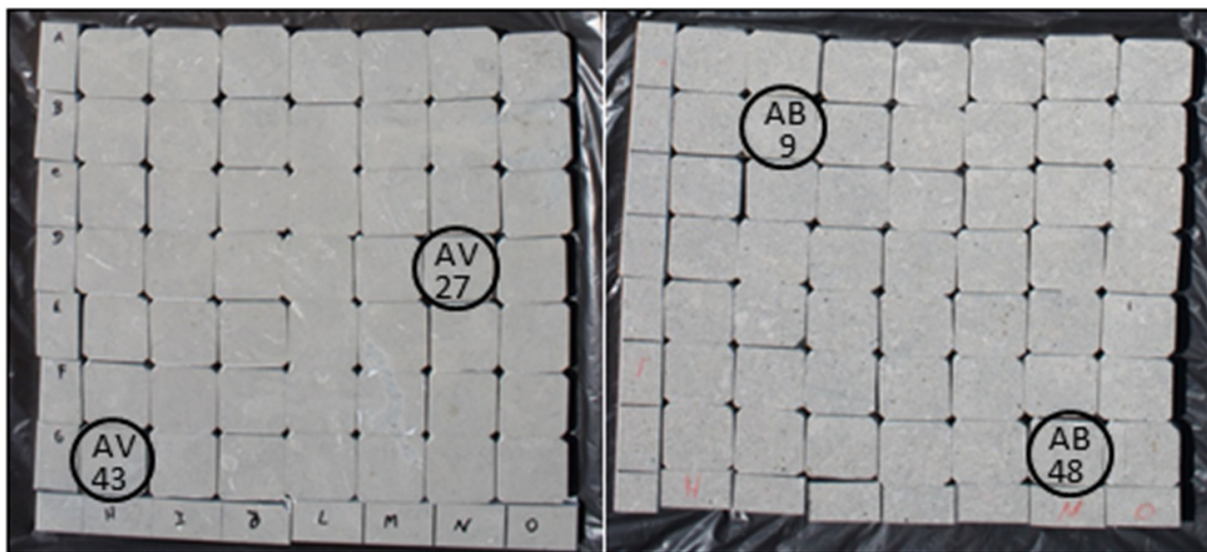
Figure 4. Azul Valverde (AV) and Atlantic Blue (AB) polished limestone fragments subject to atmospheric conditions.
