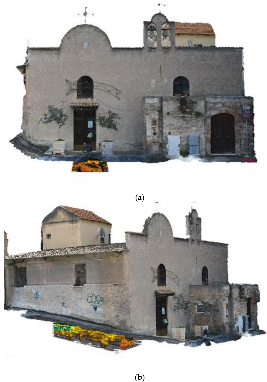
Figure 13. External 3D integration from UAV with 3D GPR built with methodology 2: (a) frontal view; (b) axonometric view.
