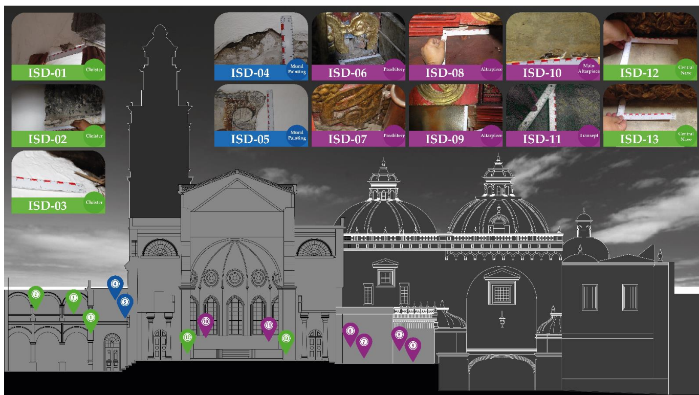
Figure 3. Blueprints of the church of Santo Domingo of Quito with the location of the analyzed samples; the figure describes the 13 samples with their locations.
