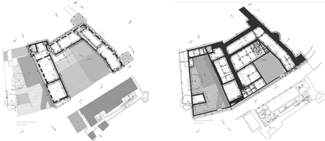
Figure 15. Two floor plan layouts obtained from the HBIM model.
