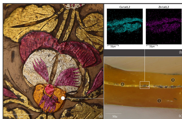
Figure 14. The lower petal, with a coppery finish, is achieved with brass leaf (a), while the iridescent whites and the golden highlights on the leaves were made with thin silver leaf. The white dot in this image indicates the sampling location (Photograph: Álvarez-White, M.C.). As can be seen in the elemental mapping (c) of a stratigraphic section (b) at 400 \times , the metallic layer (2) is an alloy of copper and zinc (Cu-Zn). Layers 1 and 3 correspond to the coloured resin layers on figure (c) (Analysis and photograph: Fernández, M.O).
