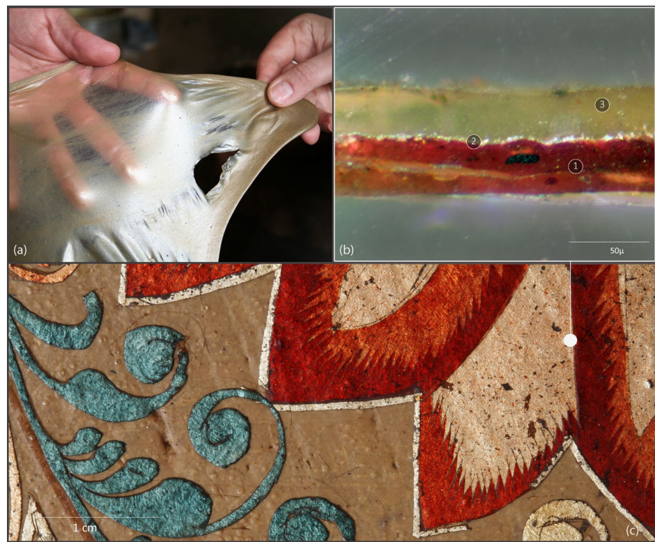
Figure 10. The delicate membranes of resin described in the 18th century are made in a similar way today (a). In the stratigraphic section (400×) (b), the yellow-tinted resin (3) layered over silver leaf (2) is visible. Layer 1 corresponds to the red-coloured resin decoration. The subtly tinted red resin membranes overlap to achieve the shading that Humboldt describes (c). The white dot in the image (a) indicates the location where the sample was taken. (Photographs (a,c): Álvarez-White, M.C) (Analysis and photograph: Fernández M.O). Private collection.
