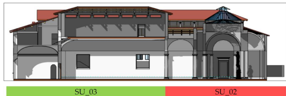
Figure 10. Longitudinal section of SU_03 ( Galleria dei Prigioni ) and cross-section of SU_02 ( Tribuna del David )—from left to right.
