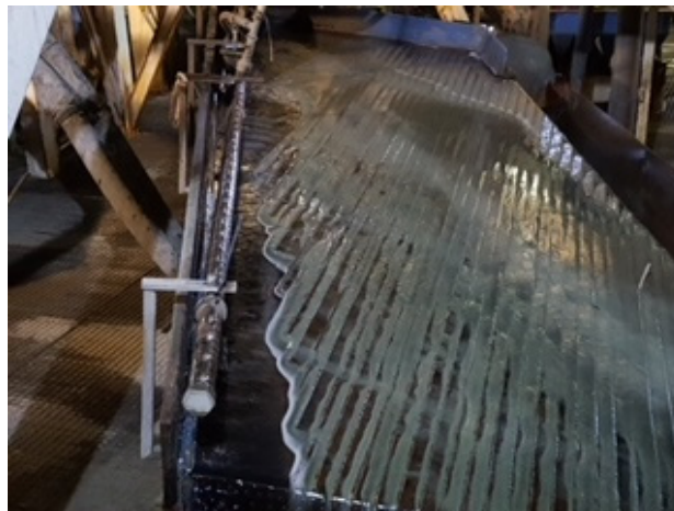
Figure 7. Flotation table used for the concentration of tungsten from mine tailings in Los Santos mine, Salamanca (Spain). Picture taken by D. Pereira.
