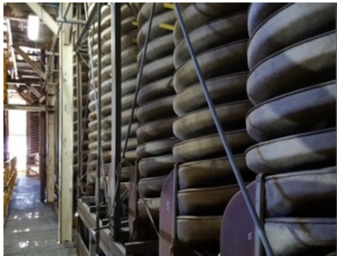
Figure 8. Inside of the infrastructure used for the separation of tungsten from mine waste in Los Santos mine (Salamanca, Spain). Picture taken by D. Pereira.
