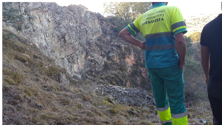
Figure 13. Mine tailings in San Pelayo. This mine waste was used to pave the road at the end of the last century and at night it is possible to detect the remains of scheelite within the gravel using an ultraviolet lamp.
