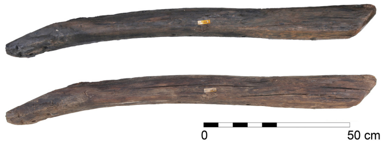
Figure 16. The condition of a frame timber before (above) and after (below) PEG impregnation vacuum freeze-drying. © YSP Archive.
