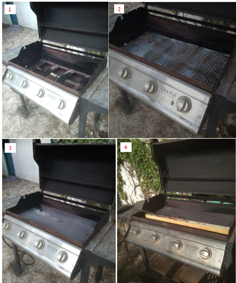
Figure 3. Commercial grill system used for heating the planks. (1) Burners are exposed. (2) Perforated sheet metal covers the flames. (3) Solid 3 mm sheet metal covers the flames. (4) Wooden plank is laid on the solid sheet metal (photo: M. Bram).
