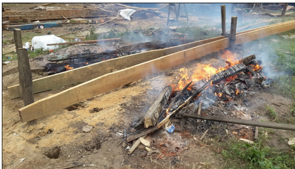
Figure 2. Heating of planks over open fire in small boatyard in Vietnam (Photo: M. Yarkowich).
