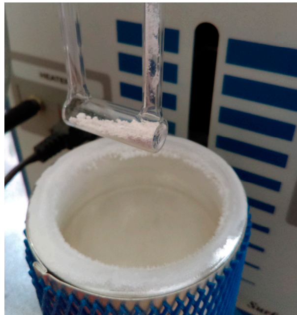
Figure 4. Horiba SA9601 STNE equipment for surface area test.
