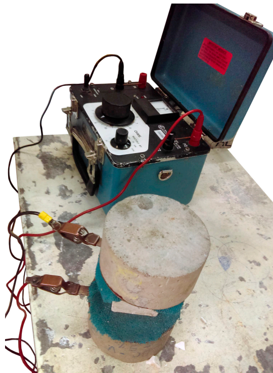
Figure 7. Electrical resistivity performance of the test.
