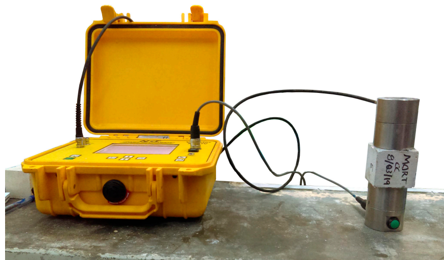
Figure 6. Ultrasonic velocity pulse equipment and testing on a sample.
