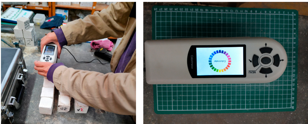
Figure 8. Utilization of the colorimetry equipment.
