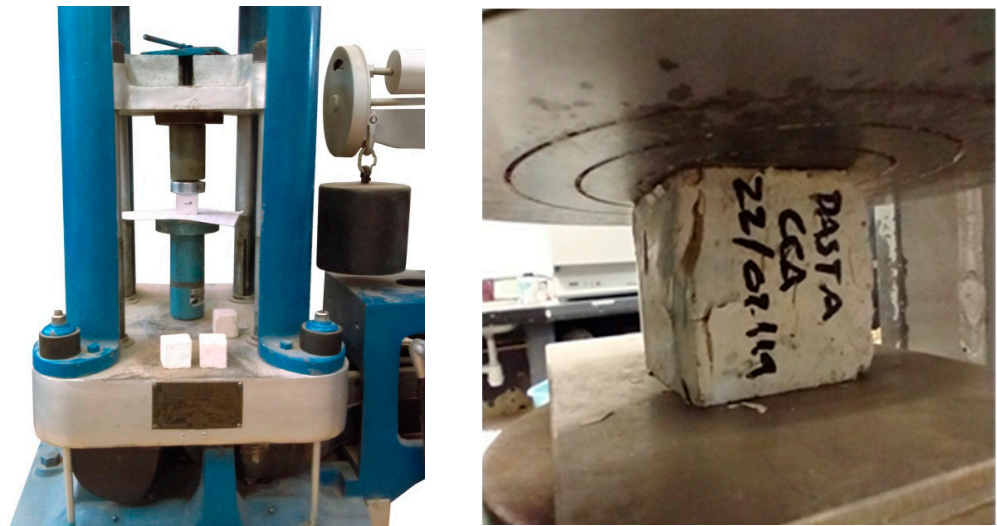
Figure 9. Universal Testing Machine and specimen failure.
