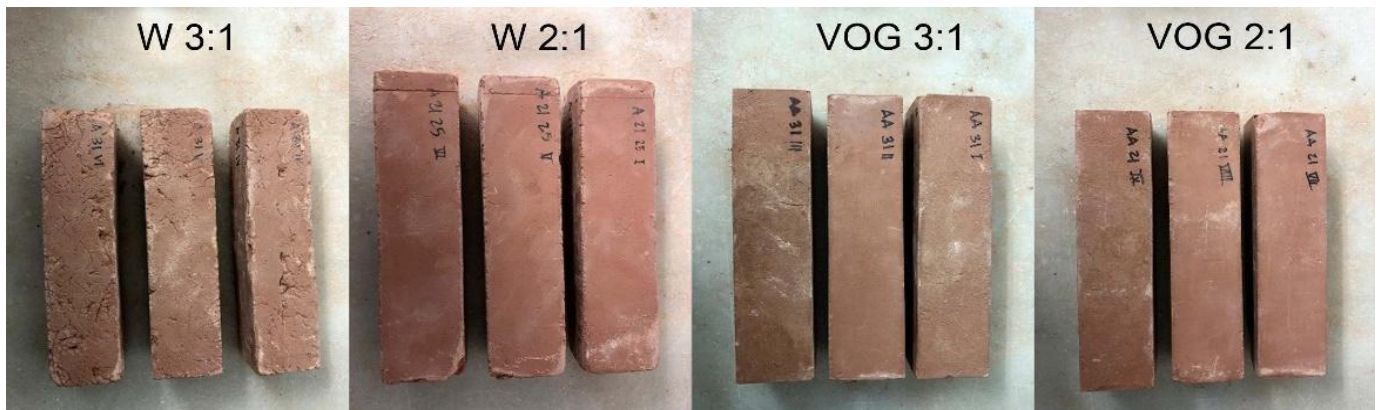
Figure 10. Specimen images after the 12 moisture-drying cycles. Source: K. Sandoval-Castro.
