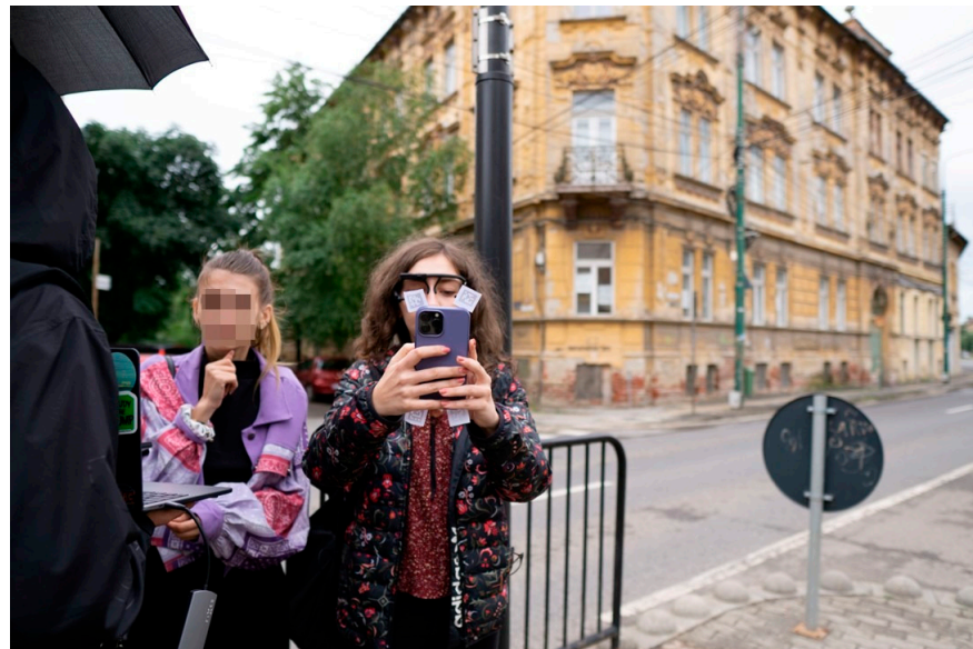
Figure 4. Markers placed around the smartphone display to calibrate the Pupil Core eye-tracking device.
