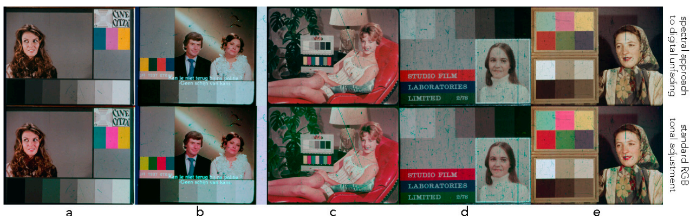
Figure 3. (a–e) Top: results obtained through the spectral approach of digital unfading. Bottom: results of a standard RGB tonal adjustment obtained with the “LUTgenerator” algorithm.
