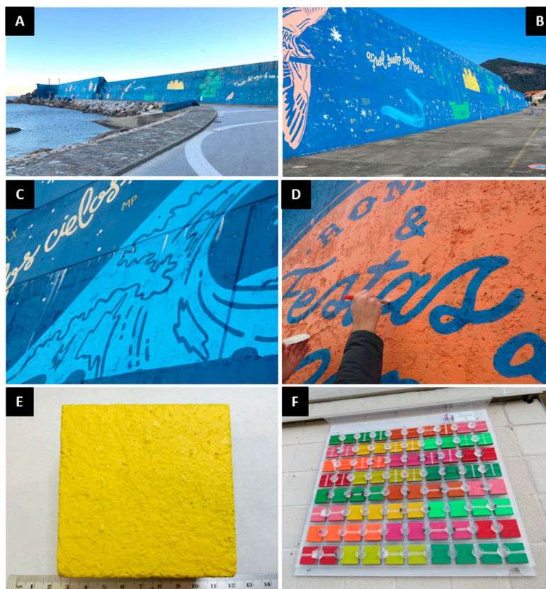
Figure 1. (A,B): different views of the A Guarda Escrita nas Estrelas mural, in which the different tones of the paints can be seen. (C): detail showing the blue base (BLB) paint on which the other paints were applied by stencilling; in this case the blue (BL) and brown (BR) paintwork can be seen; note the variable roughness of the concrete substrate. (D): application of a protector in a monitored area with orange (OR) paint. (E): concrete mock-up with yellow (YE) paint, used in the outdoor exposure test. (F): panel of mock-ups in the outdoor exposure test.
