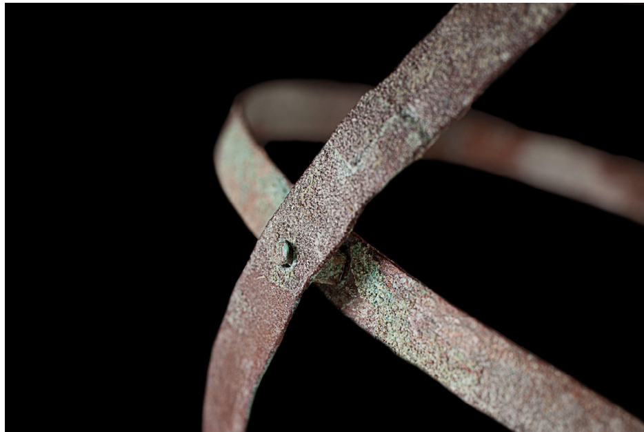
Figure 3. Detail of the mechanism articulating the gimbals. Photograph by Patricia Carrillo.
