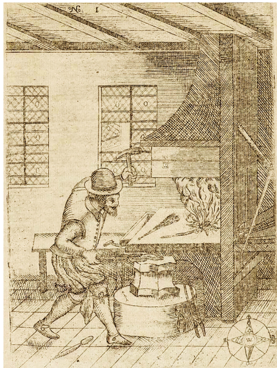
Figure 8. Image of a blacksmith hammering the tip of the lodestone, which will then be rubbed against the needle [26] (p. 137).
