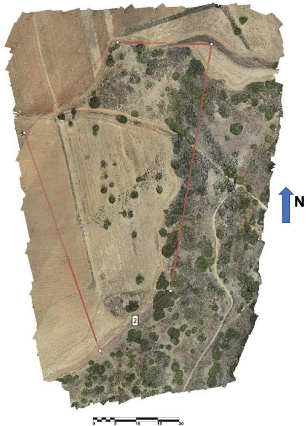
Figure 3. Shape file used to crop the orthophotos (False North), (image courtesy of the authors).
