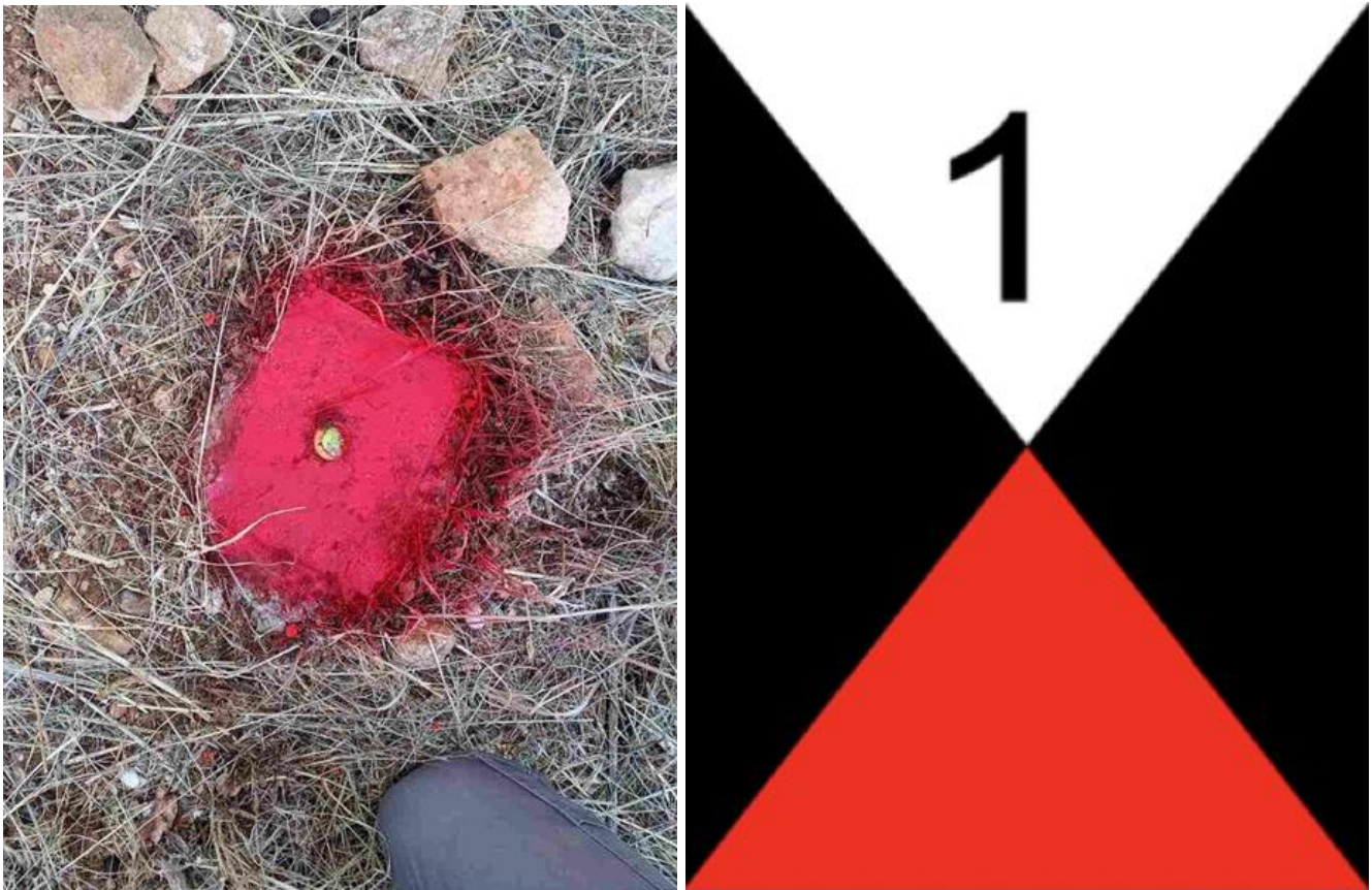
Figure 2. Permanent Ground Control Point (left) and A3 laminated targets (right), (images courtesy of the authors).
