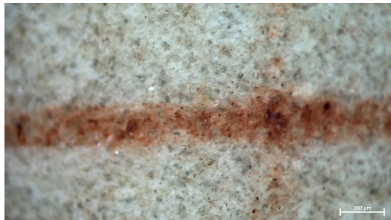
Figure S5. Microscopic image of graphic ruling in folio 20v.
