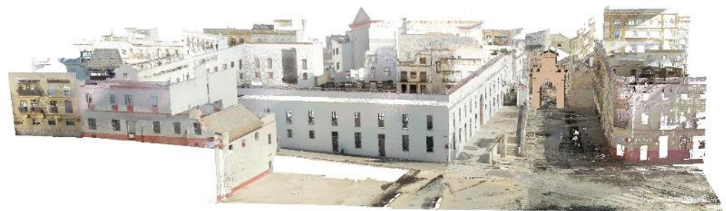
Figure 25. 3D point cloud as seen from the outside, including the location of the 3D reconstructed Puerta Real. Authors' work, 2023.
