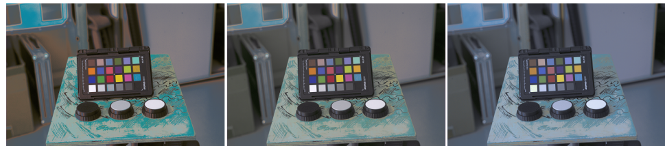
Figure 11. From left to right: calibrated sample image of the Sun set after being transformed into sRGB, Adobe RGB, and wide RGB. The multidimensional calibration function based on the saturated colours in the original picture provokes artifacts, pixelings, and miscolouring of the hues in subspaces distant to the chart values, as in the background of the image.
