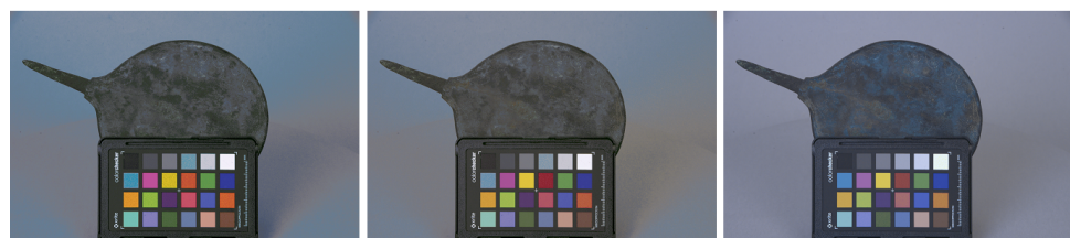
Figure 7. From left to right: calibrated sample image of the Mixed set after being transformed into sRGB, Adobe RGB, and wide RGB. It is clearly seen that the wide RGB enables the best neutralization of colour bias in the images.
