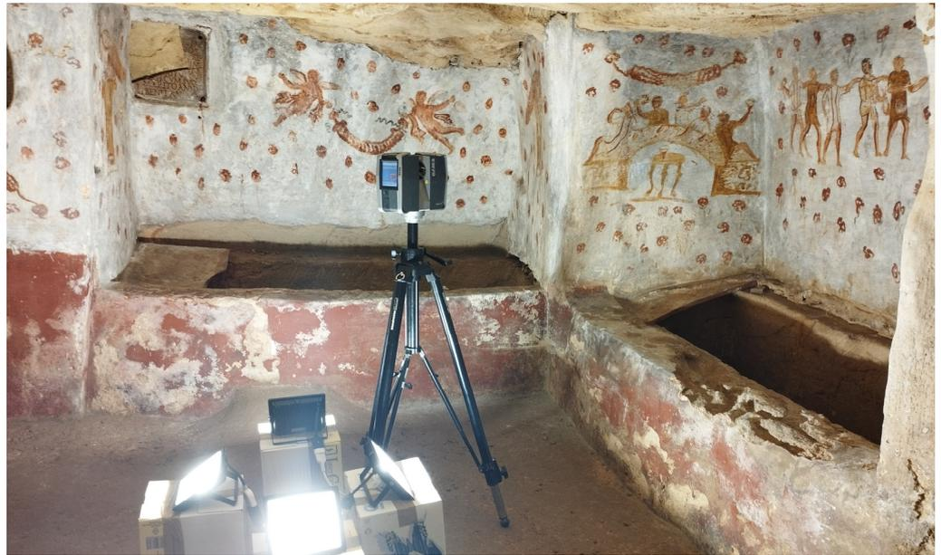
**Figure 8.** The laser scanner acquisition.
