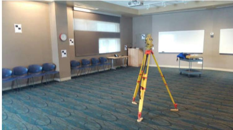
**Figure 1.** Coordinating reference targets using the total station.
