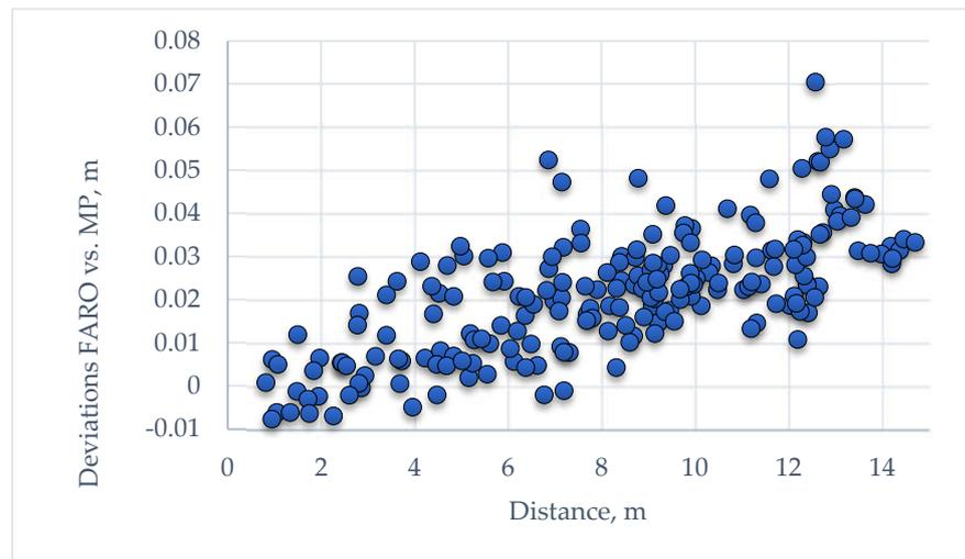
Figure 17. Distances deviations: FARO Scanner vs. Matterport.
