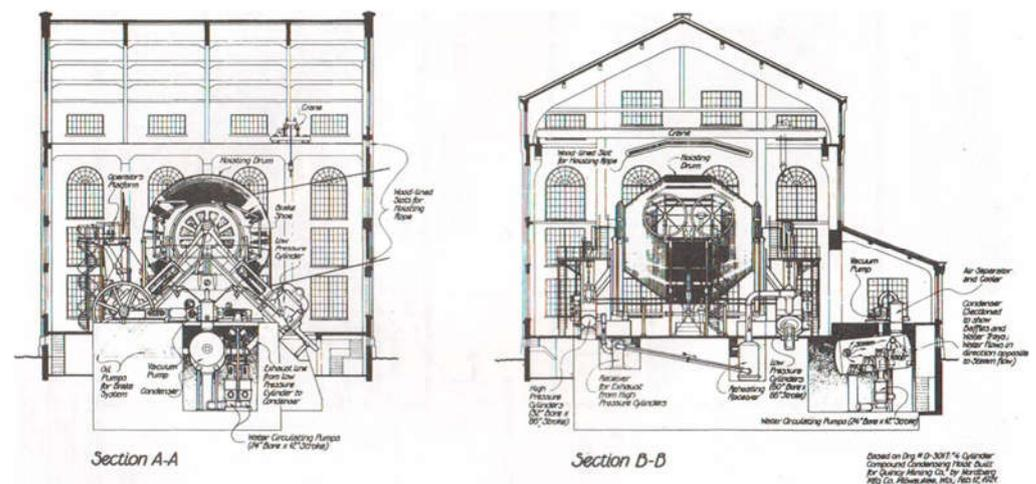
**Figure 11.** Cross-section of the Quincy Mine Hoist Engine house, 1921 (archive image) [47].
