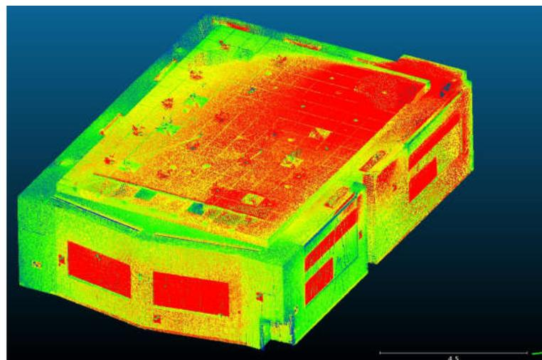
**Figure 3.** Point cloud of the test field with control targets retrieved from FARO Scanner data.
