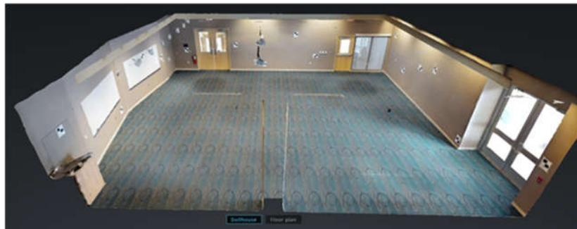
**Figure 5.** Three-dimensional model of the test field after processing by the Matterport server.
