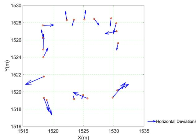
**Figure 26.** Vector plot of transformation errors in the horizontal plane.
