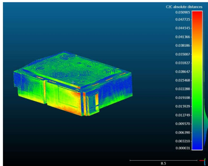
**Figure 25.** C2C distance deviations after the systematic error correction; distance units are meters. Color-scale units are meters.
