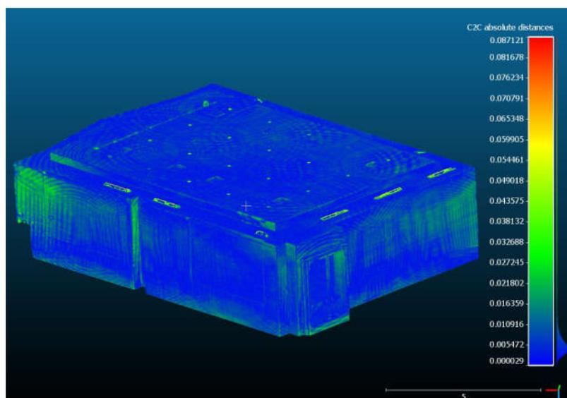
**Figure 24.** Colored 3D point cloud after blunder exclusion; distance units are meters. Color-scale units are meters.
