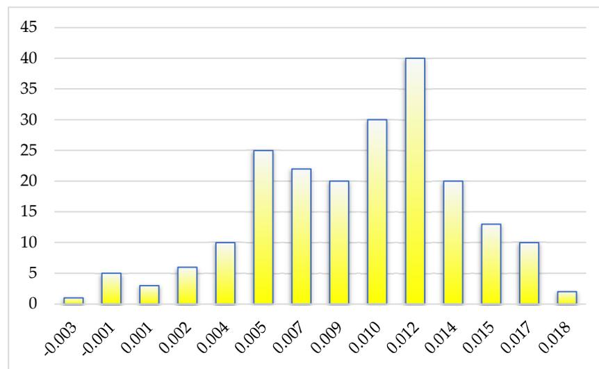
Figure 19. Histogram of deviations: Total station vs. FARO scanner.
