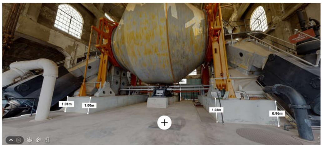
**Figure 36.** The measurements of the Hoist Engine concrete foundations in the Matterport software menu.
