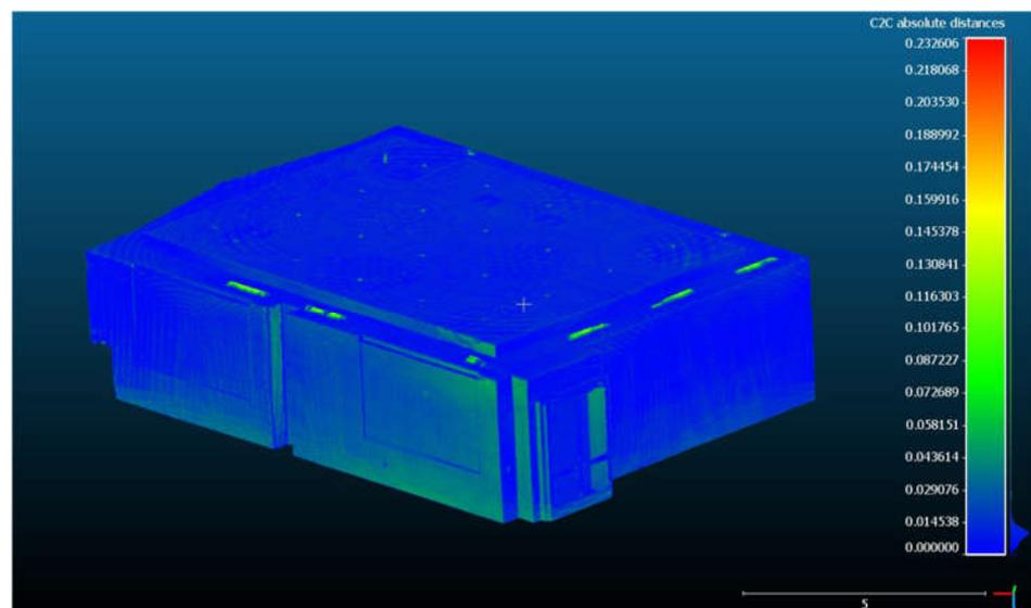
**Figure 23.** Colored 3D point cloud after C2C comparison; distance units are meters. Color-scale units are meters.
