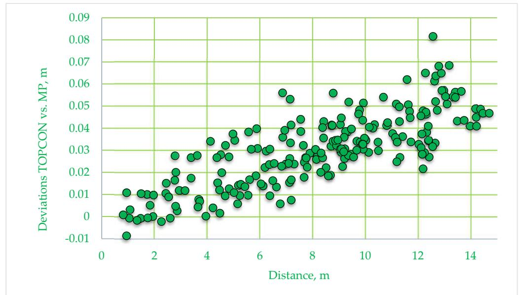
**Figure 15.** Distances deviations: Total station vs. Matterport.
