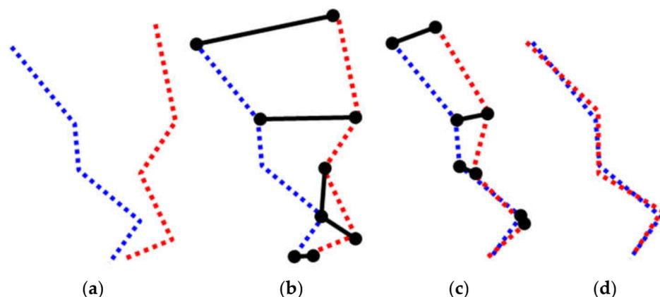
**Figure 7.** ICP orientation workflow: (a) two point clouds; (b) discrepancies determination; (c) first transformation; (d) nth transformation iteration.
