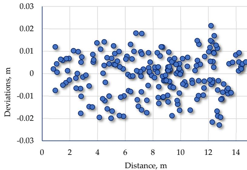
**Figure 22.** Distance deviations after linear trend correction.
