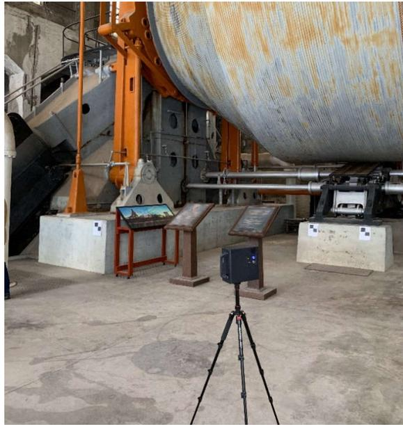
Figure 31. One of the Matterport Pro surveying stations inside the Hoist Engine house.
