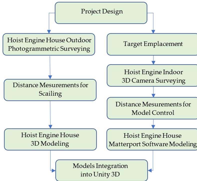
Figure 28. Flowchart of outdoor and indoor surveying of the Hoist Engine house.
