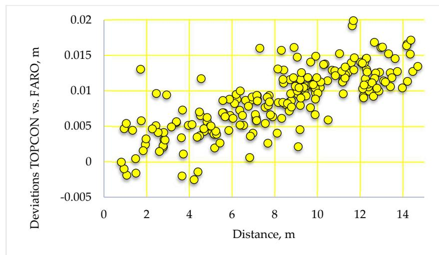
**Figure 16.** Distances deviations: Total station vs. FARO Scanner.
