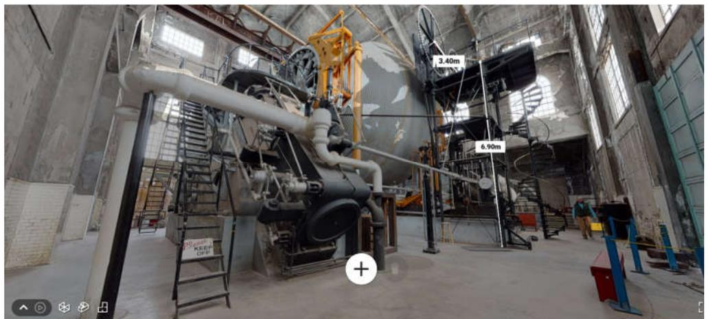
**Figure 35.** The ladder height measurement option in the Matterport software menu.
