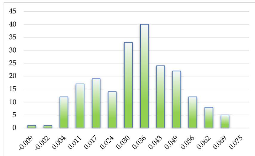
Figure 18. Histogram of deviations: Total station vs. Matterport.
