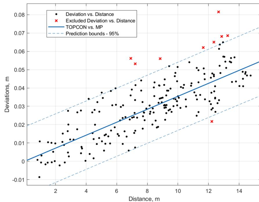
**Figure 21.** Results of the linear approximation.
