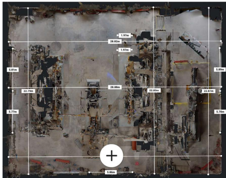
**Figure 38.** Distance measurements according to the map of the Quincy Mine Hoist Engine house.
