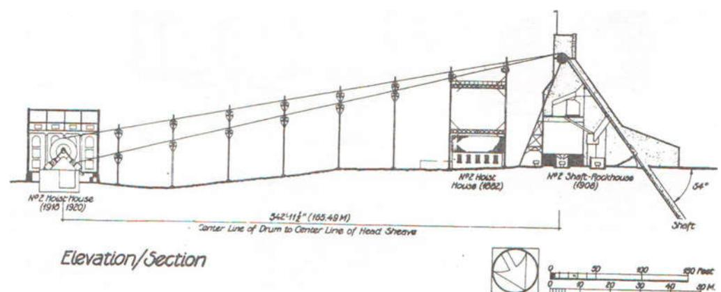
**Figure 10.** General view of the Quincy Mine, 1882–1920, with the Hoist Engine house leftward (archive image) [47].
