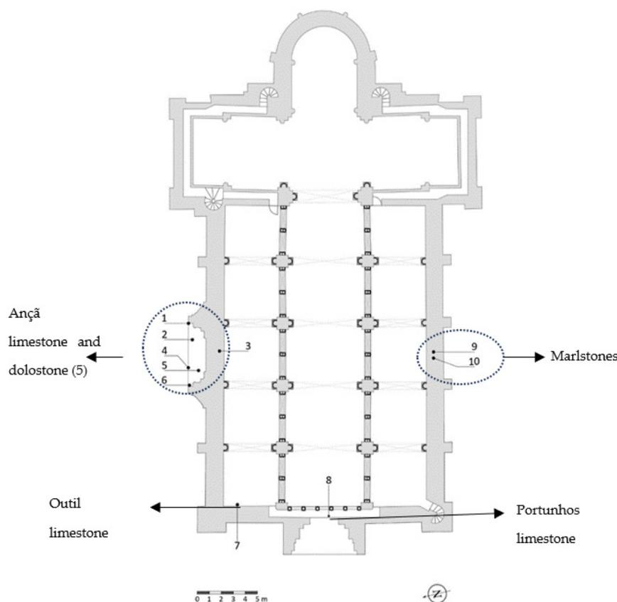
**Figure 11.** Distribution of carbonate stones (recorded from new data). 1—PEE; 2—PEch; 3—PES; 4—PEC; 5—PE1; 6—PER; 7—PLE; 8—PPch; 9—PEt; 10—P3P.
