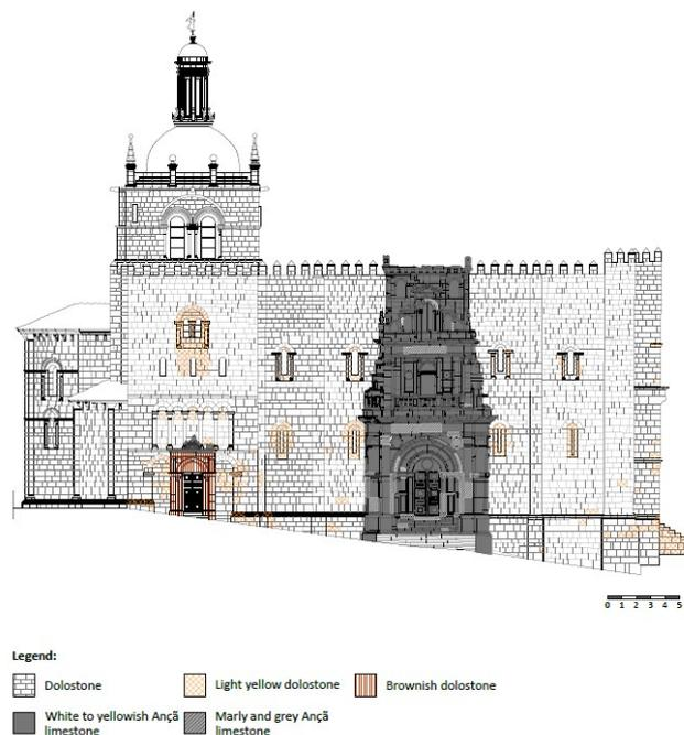
**Figure 4.** Mapping of stones from North facade of Coimbra's Old cathedral (based on the LNEC drawing) [16].
