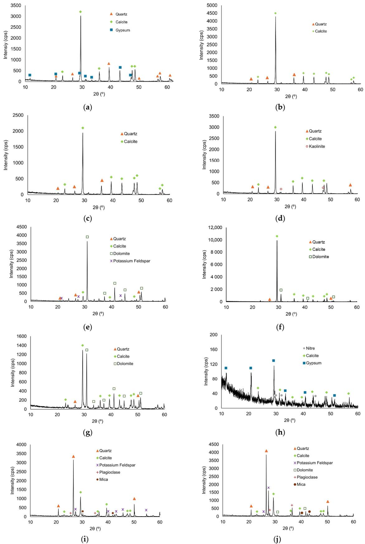
**Figure 8.** XRD graphs obtained: (a) PES; (b) PEC; (c) PEE; (d) PER; (e) PPch; (f) PLE; (g) PE1; (h) PEch (i) PET; (j) P3P.
