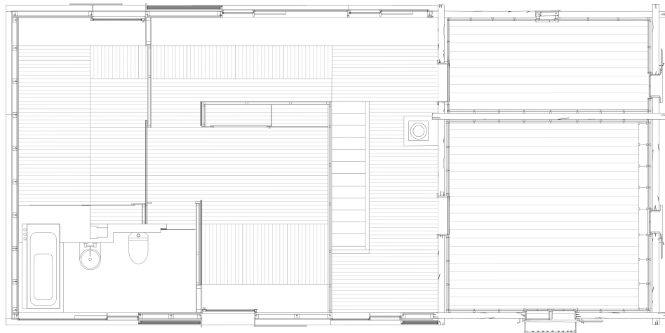
Figure 31. Gugalun House. The plan of the first floor. Note the arrangement of the floor planking that solves the timber framing of the floor slabs. Studio Adam Caruso, ETH Zurich (Simon Burri, Grégoire Farquet, Michael Fehlmann, and Lea Hottiger).
