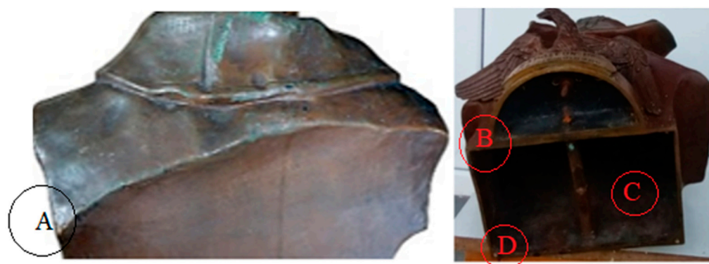
Figure 6. Areas where sampling was performed: (A)—left shoulder, back; (B)—the base of the plinth (support–pedestal); (C)—the surface of the inner cavity of the statue; (D)—the bracket or statue’s shoe fixing screw.
