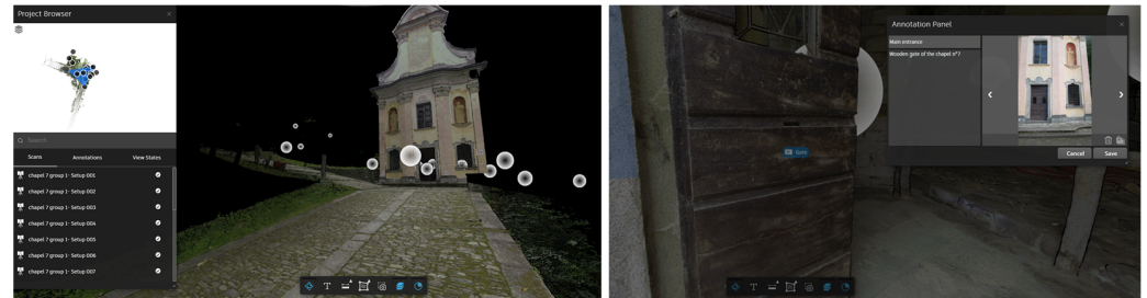
Figure 3. An example of use of the Autodesk Drive platform, showing the navigation of the point cloud through the scan positions (gray circles), and the use of annotation function for information and media attachment. Dataset from [1].
