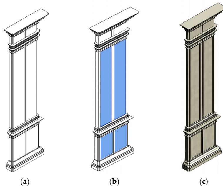
**Figure 16.** The main parts of the pillars: (a) shaft and pedestal at the end of the extrusions, (b) the void extrusion on the shaft for carving its section, (c) a rendered model of the whole double pillars.
