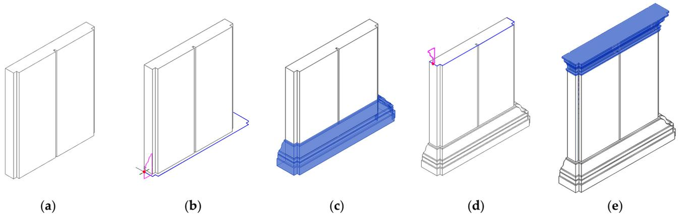
**Figure 15.** Different operations to obtain the pedestal of the double pillars and its mouldings: (a) extrusion of the main body, (b) generation of the lower moulding's profile (c) its extrusion on a path, (d) generation of the upper moulding's profile (e) extrusion on a path.
