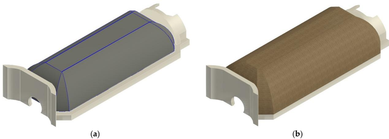
**Figure 19.** The strategy followed for modelling the boat vault of the main nave: (a) the initial mass overlaid to supporting structures of the model, (b) the actual roof obtained from the command “Roof from mass” according to its constructive layers.
