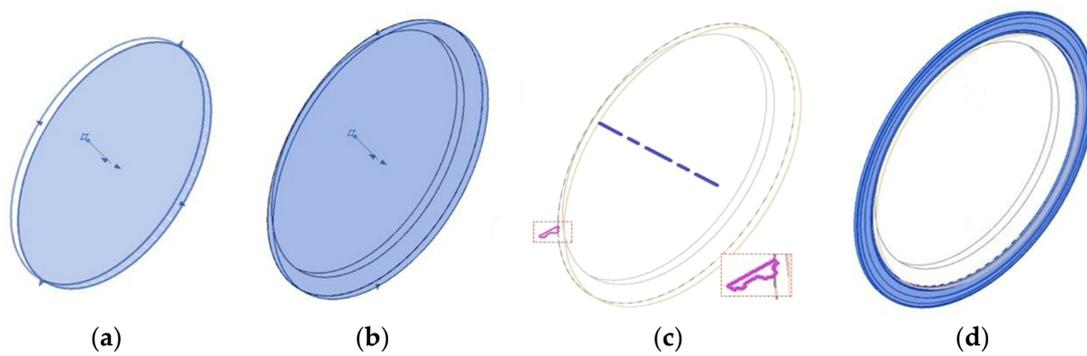
**Figure 17.** The sequenced process to obtain the rose window: (a) the cylindrical void cutting the wall, (b) its splays on façade and counterfaçade, (c) the extrusion of the annular moulding on a circular path on the counterfaçade, (d) the rose window at the end.
