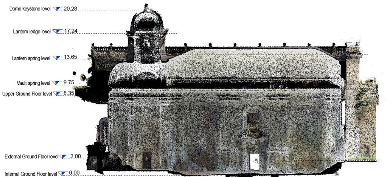
**Figure 12.** Main reference levels for parametric modelling.
