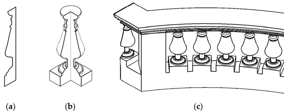
**Figure 20.** The modelling process for the parapet: (a) the generative profile of the stringer, (b) the revolution of the profile on its vertical axis, (c) the alignment of the offset stringers along the top perimeter of the building.
