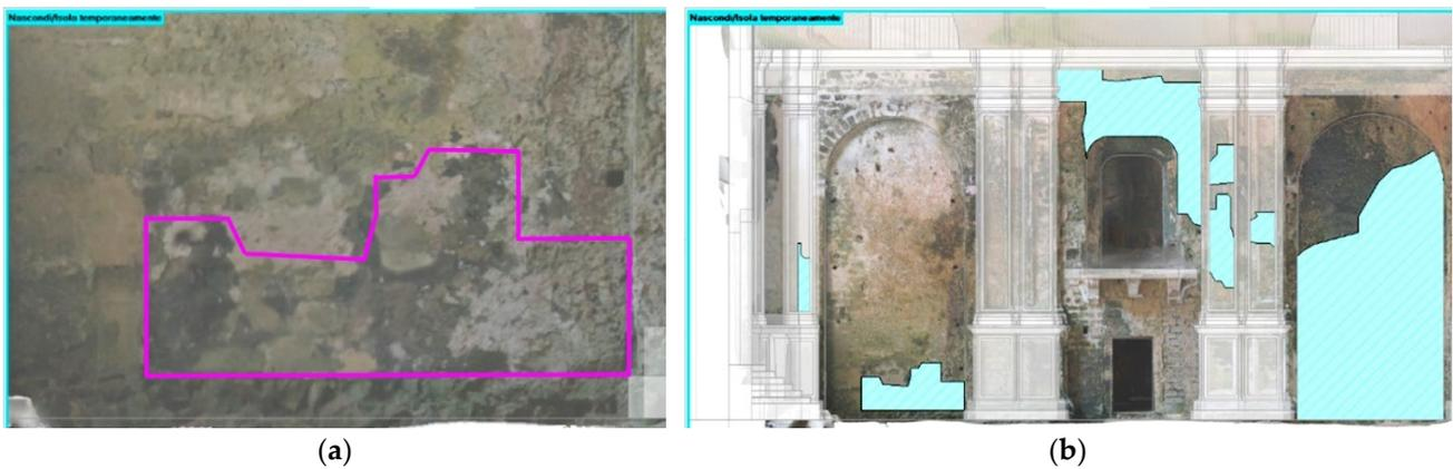
**Figure 23.** An example of contour tracing: (a) detail of fragmentation on surface layer; (b) the parametric families created accordingly.
