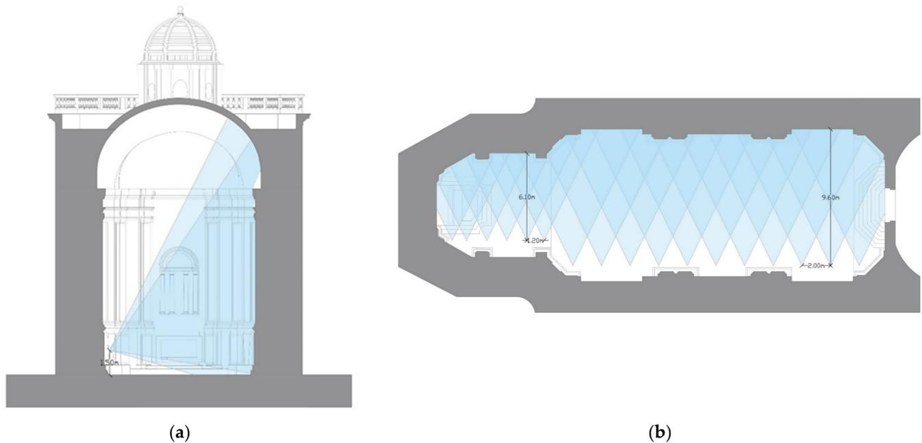
**Figure 9.** Scheme of the terrestrial photogrammetric survey of the internal façades: (a) in section, (b) in plan.
