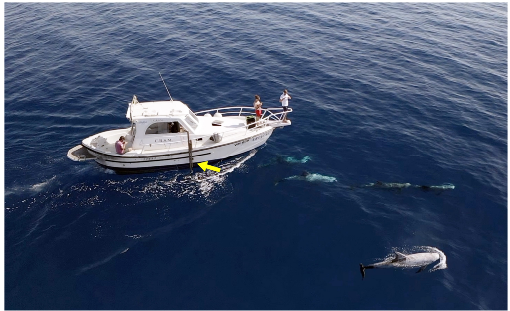
Figure 3. The boat ARPACAL (Regional Agency for Environmental Protection—Calabria) used to carry out the SBP surveys. The arrow indicates the instrument’s “pole” arrangement on the side. Some curious dolphins participate in the survey activities (photo by F. Mauri).
