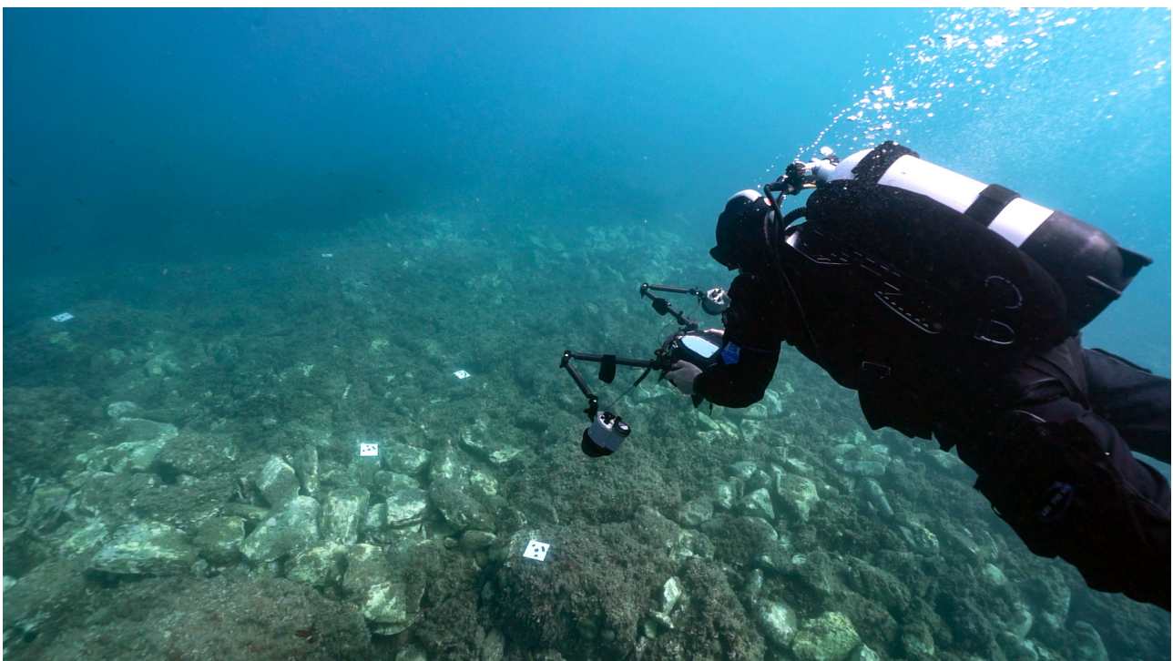
Figure 27. Le Castella. An underwater operator carrying out the 3D optical survey of Figure 23.
