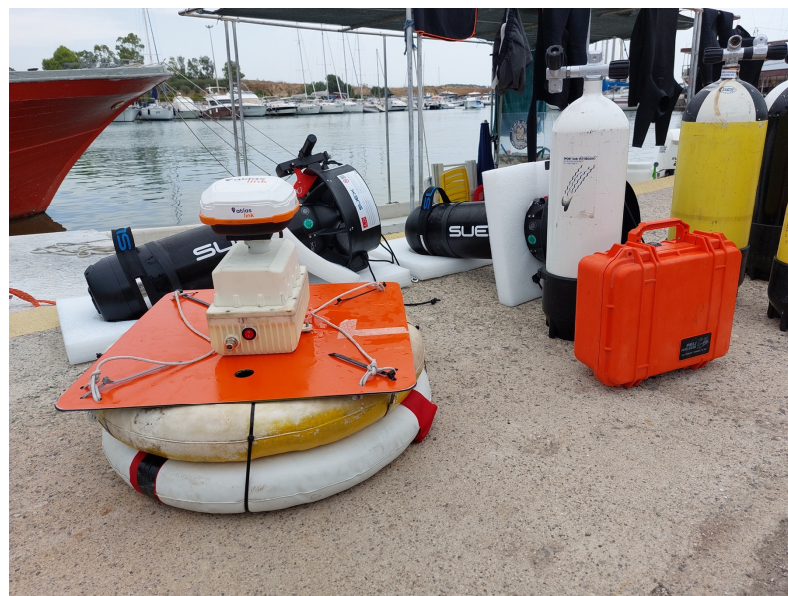
Figure 6. Artificial atoll with GPS Atlaslink™ GNSS Smart Antenna.
