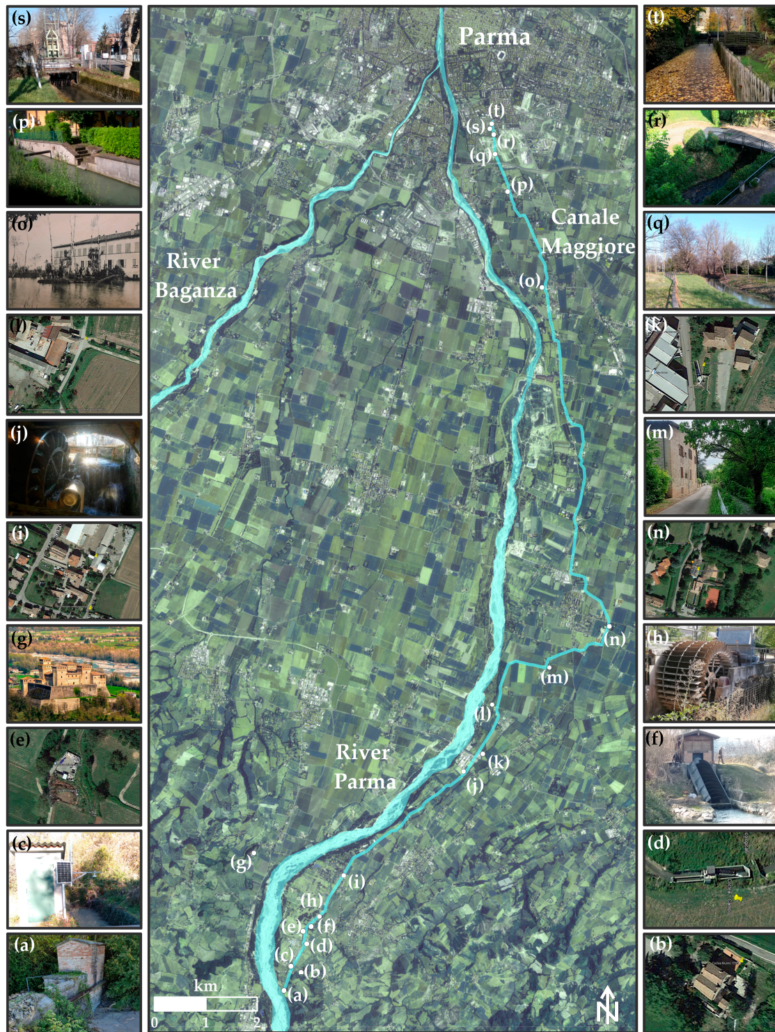
Figure 6. Sites of interest along the course of the Canale Maggiore: (a) intake structure, (b) mill dated 1555, (c) real-time stream gauging station, (d) first Archimedean screw turbine (AST) in Lesignano de' Bagni, (e) Lesignano de' Bagni waste collection area, (f) second AST in Lesignano de' Bagni, (g) Torrechiara castle, (h) water wheel at the Oasi Bianca farm site, (i) abandoned area in Lesignano de' Bagni, (j) water wheel at the Mulino di Sopra restaurant, (k) AST in Mamiano, (l) mini hydro plant site in Mamiano, (m) route along the canal in Basilicanova, (n) Mulino di casa Sforza restaurant, (o) old postcard of the lake at the Porporano paper factory, (p) stairway to access the canal in Mariano, (q) Eurosia Park in Parma, (r) glimpse of the Canale Maggiore in a private garden, (s) trash rack cleaning machine, and (t) the Canale Maggiore in Bizzozero Park in Parma.
