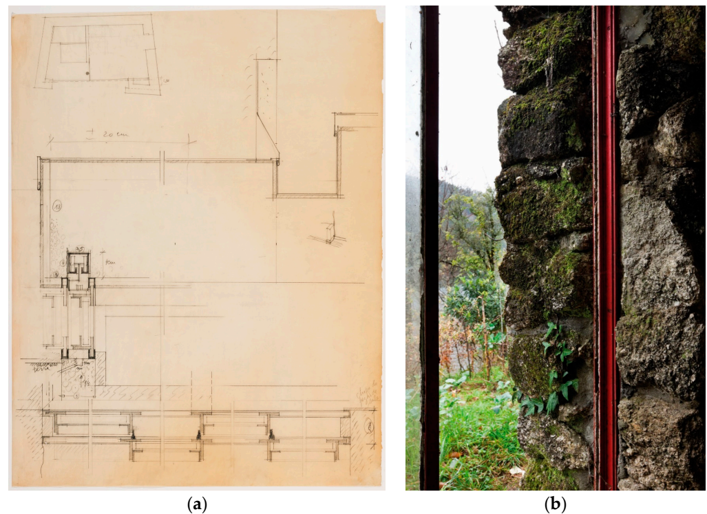
Figure 20. Eduardo Souto de Moura: House in Gerês (1980–1982). Constructive detailing: (a) drawing of the window frames (source: Eduardo Souto de Moura); (b) view of the encounter between the stone wall and the glazing profile (source: Luís Ferreira Alves).
