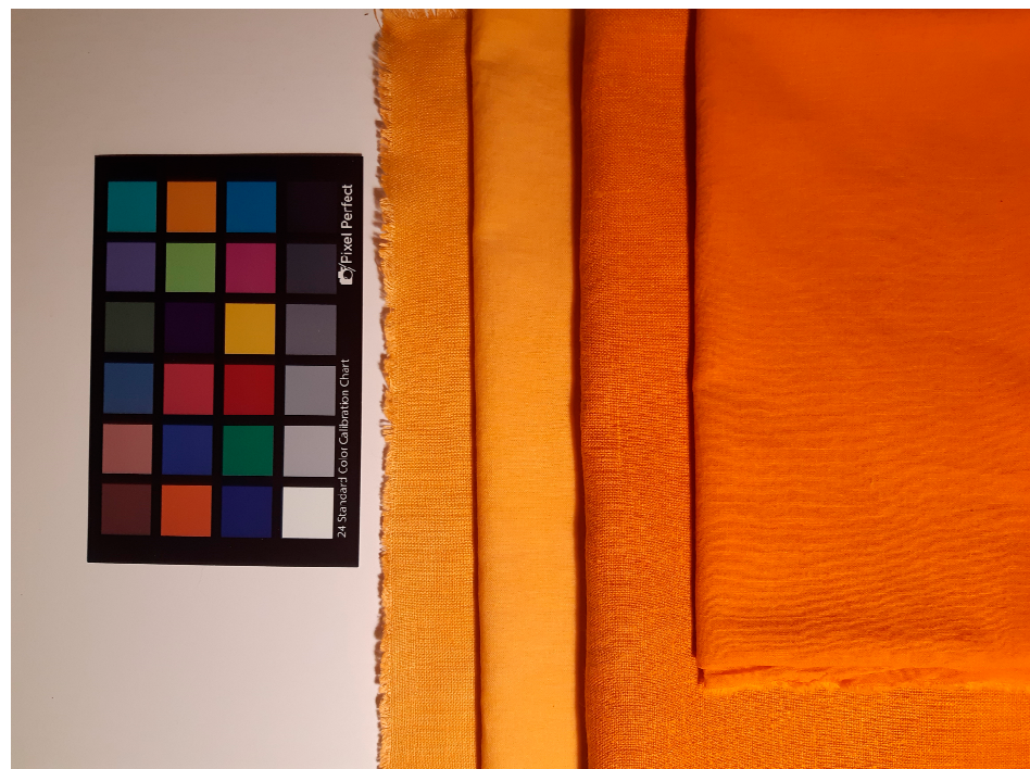
Figure 10. Fabric samples dyed with Bixa orellana L. From the left: (1) linen fabric and (2) cotton fabric dyed in a liquid obtained by soaking the plants producing the dyestuff in water. Next: (3) linen fabric and (4) cotton fabric dyed in a liquid obtained by soaking the plants producing the dyestuff in an alkaline solution.
