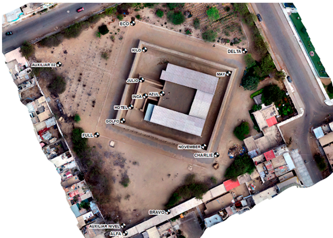
Figure 3. Establishment control points and vertical control point location for compound geometric leveling of closed traverse.
