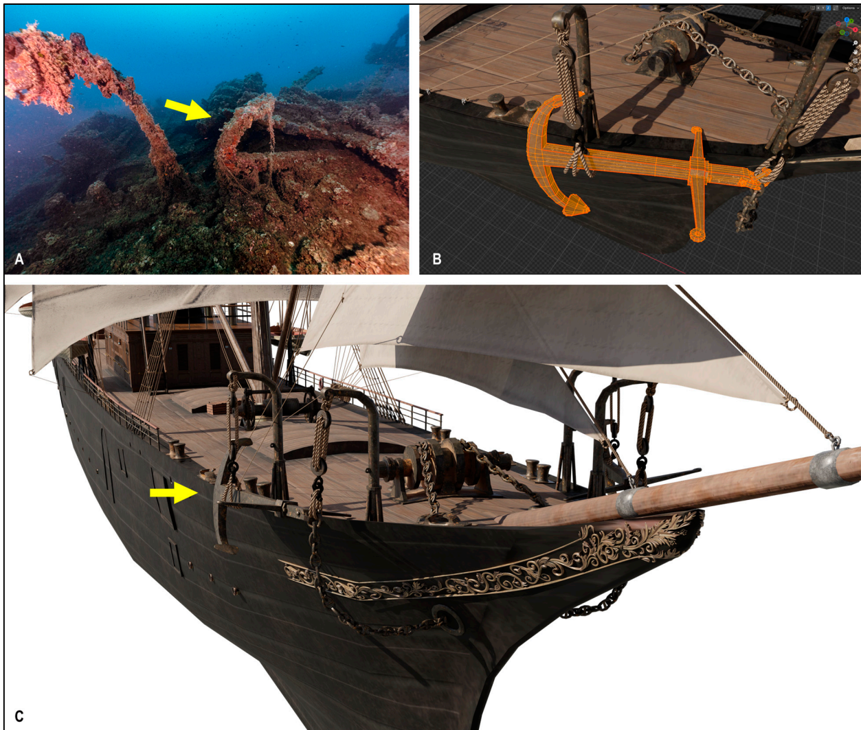
Figure 20. (A): One of the two bow anchors still in place; (B): admiral's anchor: selection in Edit Mode of Blender; (C): view of one of the anchors secured to the davits (elab. F.F., M.C., S.M., and R.P.).
