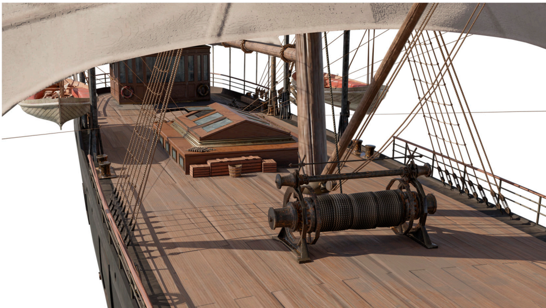
Figure 19. Three-dimensional model of the steamship Bengala : view of the upper deck with the windlass positioned below the main mast and, further aft, the butterfly hatch (elab. R.F.).
