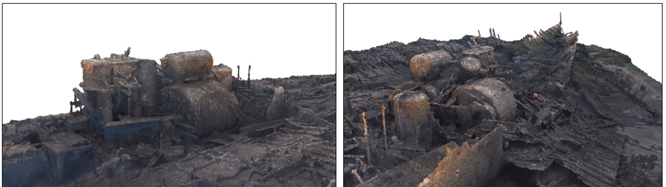
Figure 4. Wreck sector with remains of the steam propulsion system. Images extracted from the 3D survey mesh (elab. M.C. and F.F.).
