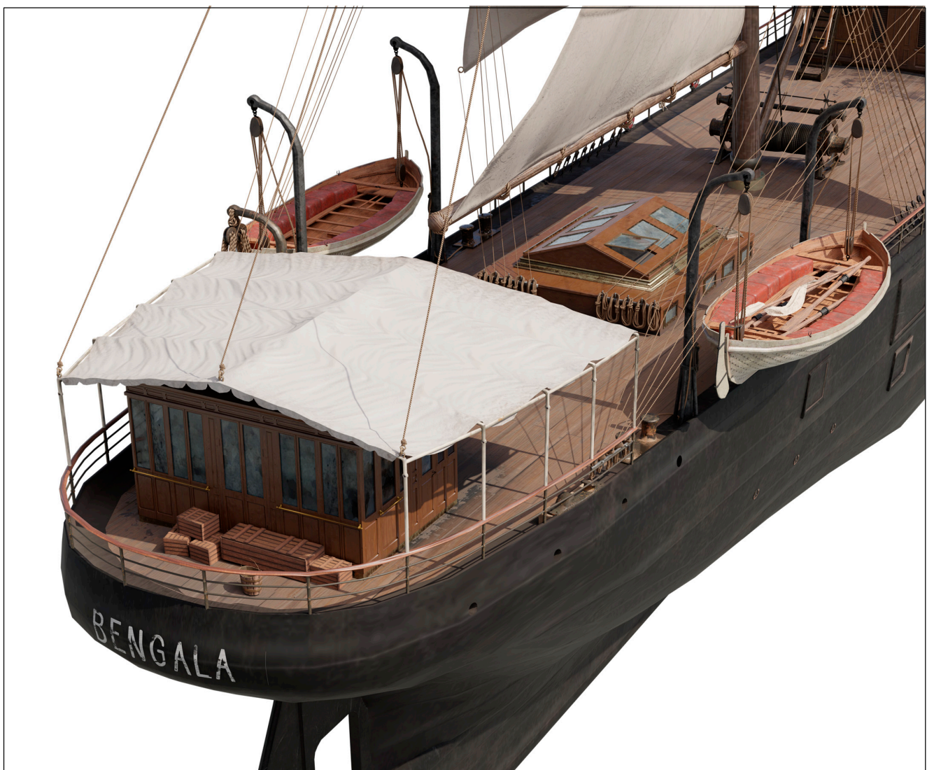
Figure 16. Three-dimensional model of the steamship Bengala : view of the stern with the roundhouse and the canopy above (elab. R.P.).
