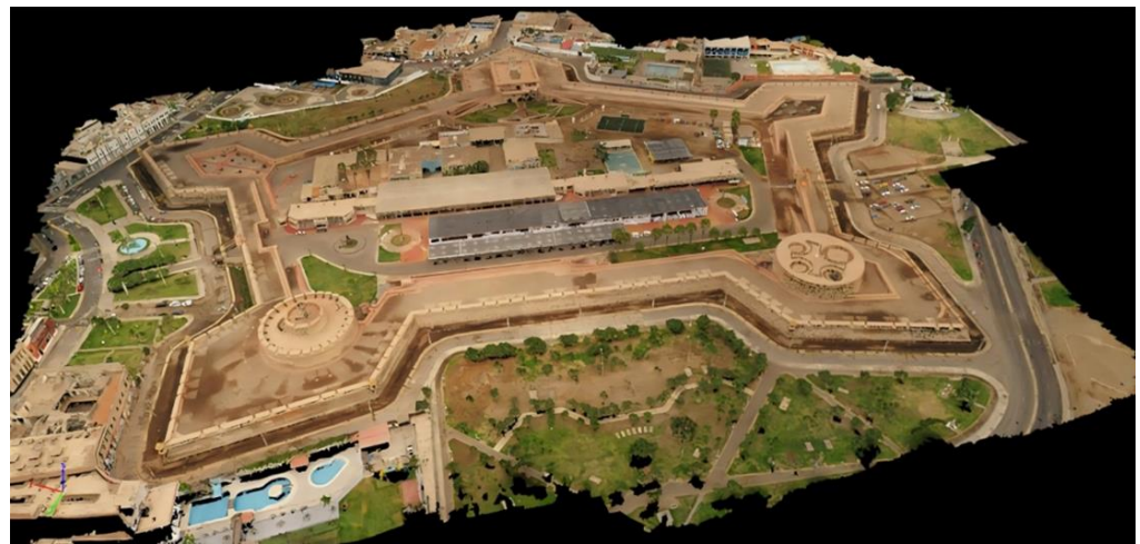
Figure 4. Three-dimensional (3D) model of the fortress generated from photographic data using PIX4Dmapper software https://www.pix4d.com/product/pix4dmapper-photogrammetry-software/ (accessed on 7 January 2025).
