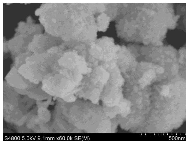
Figure.S2 The SEM of the mix sample for \text{SnO}_2 and \text{Sb}_2\text{O}_3 nanomaterials
