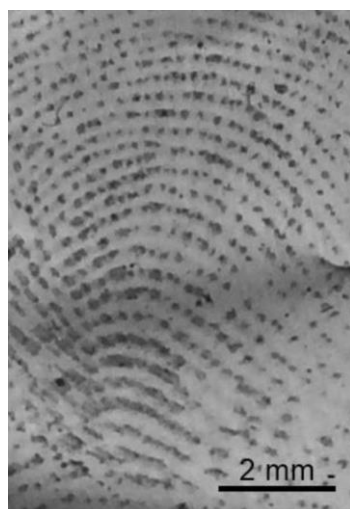
Figure 5. Photography under white light of a latent fingerprint from a 29-year-old female donor deposited on aluminum foil and treated with the green synthesized AgNP suspension for 24 h.
